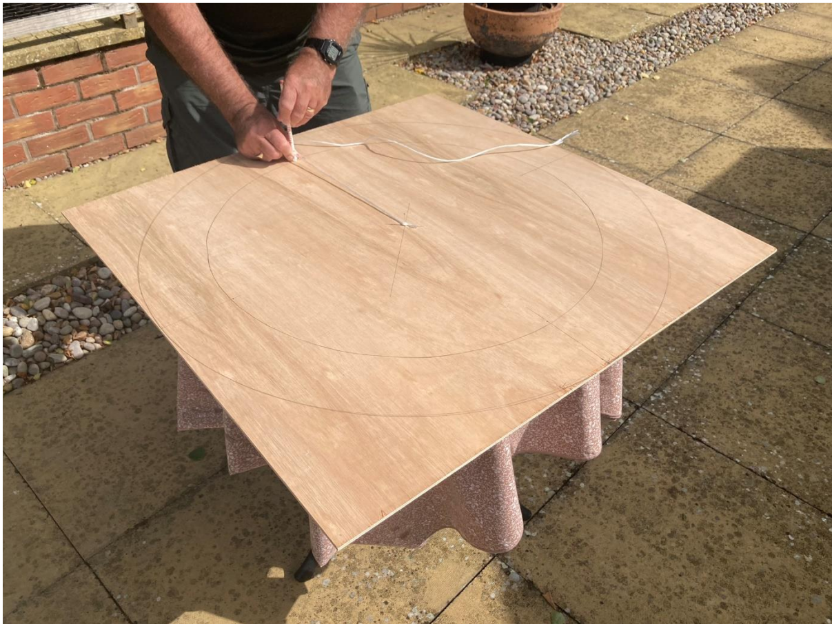
Figure 4 - Marking the Track Bed
