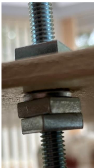
Figure 35 - Locking the Bottom Bolts
