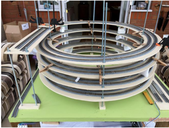
Figure 30 - Gluing the Track
