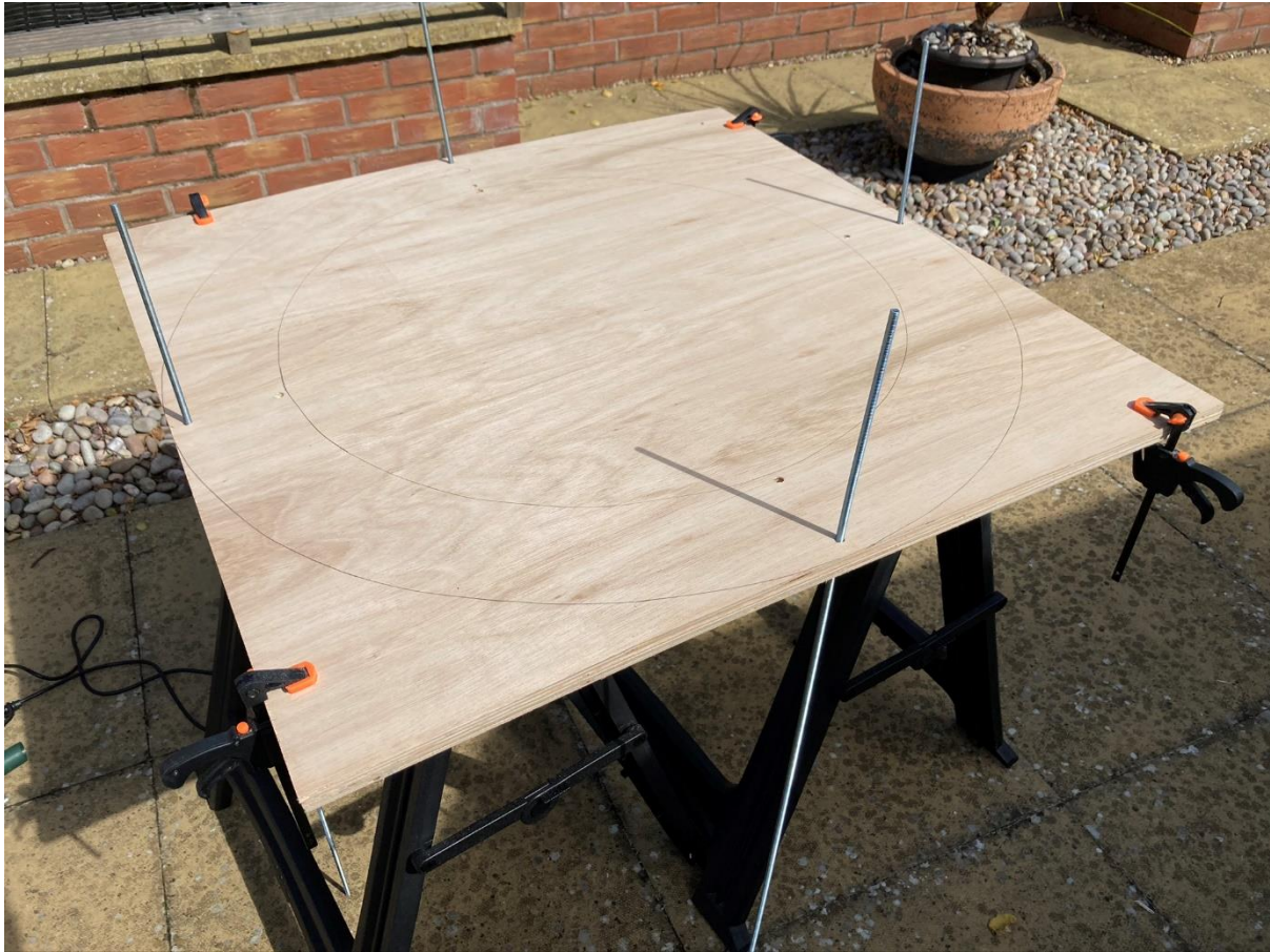
Figure 7 - Aligning the Cutting Set Before Sawing
